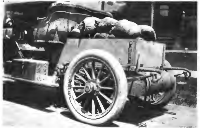
1,000-lb. Load of Wet Sand Carried in Stearns Car Tests
